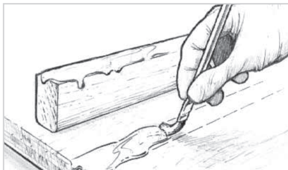
Figure 16-8 Wet out bonding surfaces with unthickened epoxy for maximum penetration and greater adhesion.
