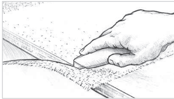
Figure 16-19 Trim excess cloth after the epoxy has begun to gel using a sharp utility knife.
