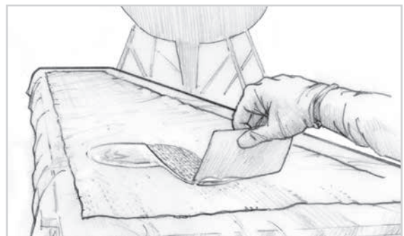
Figure 2 Wet out the fabric by pouring epoxy onto it and spreading it out with a plastic spreader
