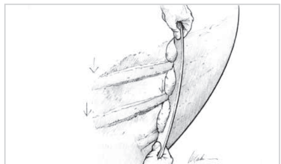
Figure 14-12 Drag the batten along the guides, removing excess mixture and leaving the surface between the guides smooth and level with the
