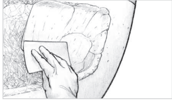
Figure 12-12 Wet out the repair surface with unthickened epoxy. Figure 12-13 Apply a layer of epoxy/406 thickened to a mayonnaise consistency.
