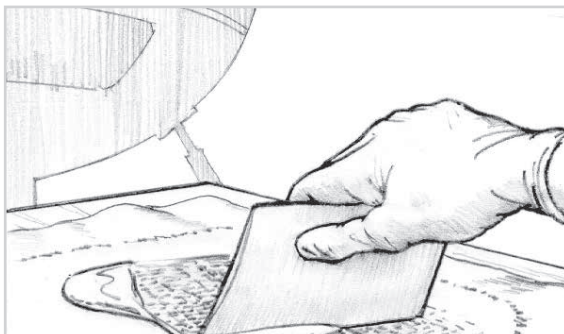
Figure 12-14 Wet out each piece of cloth with unthickened epoxy and squeegee into place.
