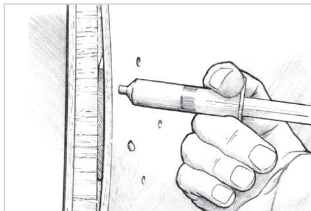
Figure 5-1 Inject epoxy under the skin using an 807 syringe with the tip cut off to match the hole diameter.
