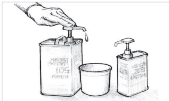
Figure 16-4 Dispense the proper proportions of resin and hardener. Figure 16-5 Stir resin and hardener together thoroughly, at least one minute—longer in cooler temperatures.
