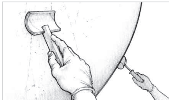
Figure 15-2 Tip off each batch, as soon as it is applied, by dragging a roller cover brush lightly over the wet surface.
